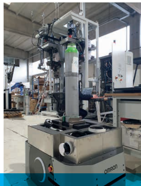
Logistica interna con navette AMR In-house logistics with AMR shuttles
