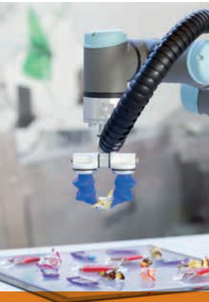
Pinza adattativa industria del food // Adaptive gripper for food industry
