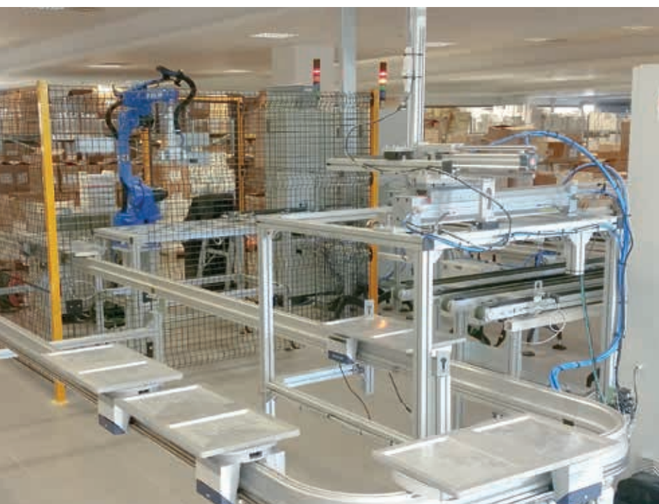
Logistica interna con navette shuttle su guide In-house logistics with shuttles on guides
