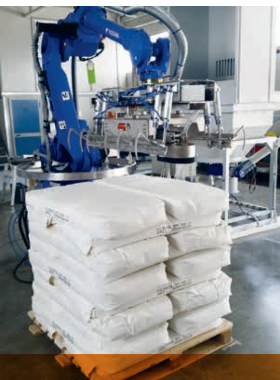
Depalletizzatore, taglia e svuota sacchi Depalletizer, cutting and emptying bags in chemical and food industry
